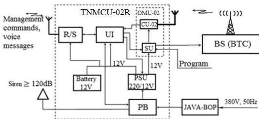
Figure 2 – Block Diagram of Radio-controlled TNMCU-02R
