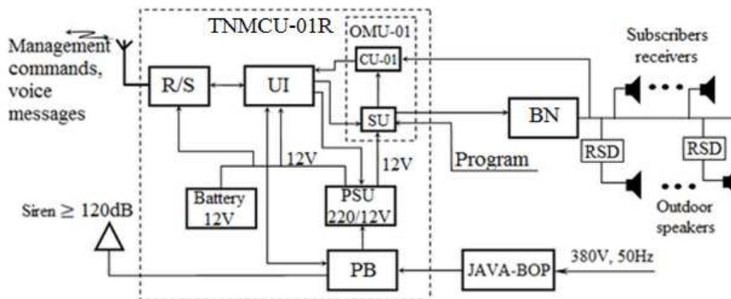
Figure 1 – Block Diagram of TNMCU-01R
