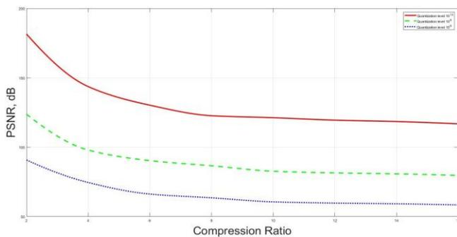
Fig. 4. The PSNR dependence on the compression ratio in the Fourier transformation
