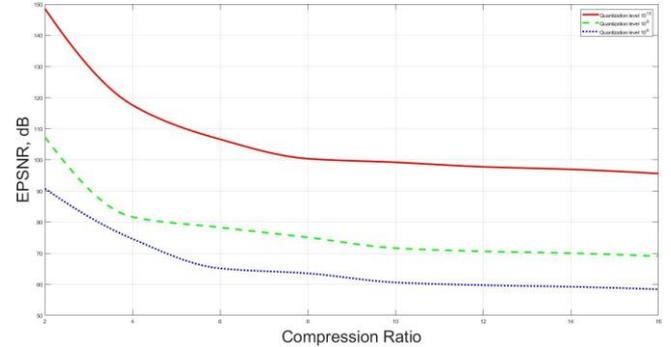
Fig. 5. The EPSNR dependence on the compression ratio in the Fourier transformation
