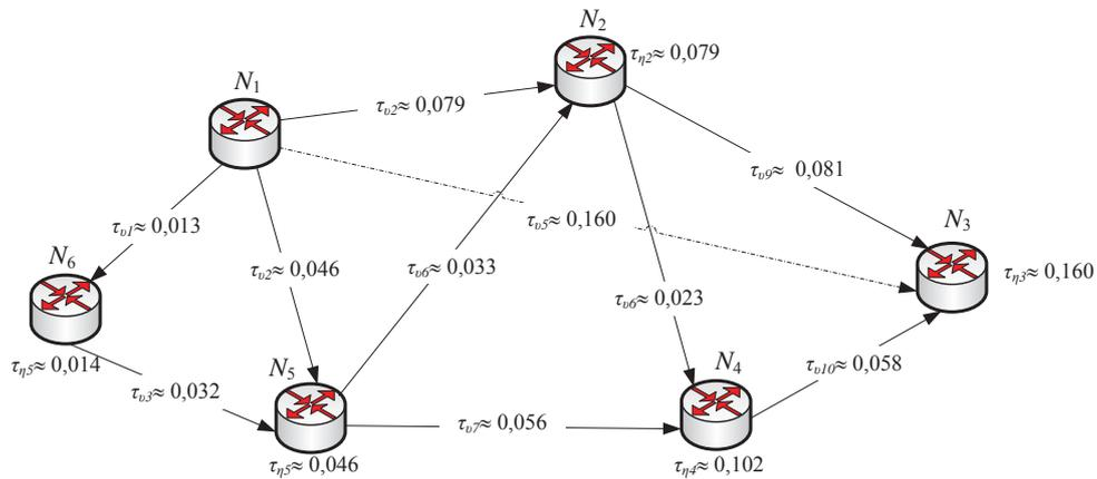
Figure 2: Results of packets delay calculations in the network without bypass routes of traffic transmission.
