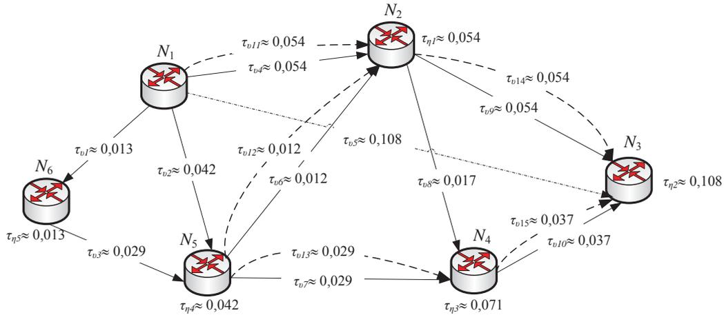
Figure 4: Results of calculations of packets delay time in the network with bypass routes of traffic transmission.
