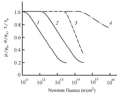
Fig. 3. The changes of the relative values of the n-type silicon parameters after the irradiation of neutrons with an energy of  $\sim 10$  keV: 1 – the lifetime of nonequilibrium charge carriers  $\tau / \tau_0$ ; 2 – the concentrations of the majority charge carriers  $n / n_0$ ; 3 – the concentrations of the majority charge carriers  $n / n_0$ ; 4 – mobility  $\mu / \mu_0$ . The value of the lifetime before irradiation is  $\tau_0$ , s: 1 –  $10^{-6}$ , 2 –  $10^{-9}$ .
