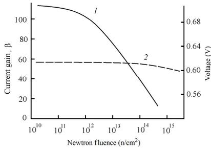
Fig. 2. The dependences of current gain of common-emitter circuit  $\beta$  (1) and voltage on the emitter p-n-junction  $U$  (2) on the neutron fluence
