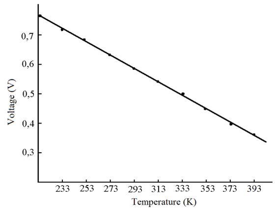
Fig. 1. The dependence of the forward voltage on the emitter p-n-junction of the BJT on the temperature at a current value of 100  $\mu$ A
